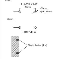
3. Use M6 screws to install the pole onto the wall. (Ensure screws are tightened.)
